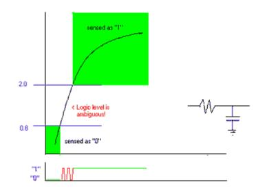
Due to the slow rate of voltage change, the signal remains in the "gray zone" too long, so it may be interpreted as shifting ON and OFF instead of changing smoothly from one logic level to the other. If one is attempting to count the input or take some action when it changes state, this can be disastrous. There are several ways to deal with this:
